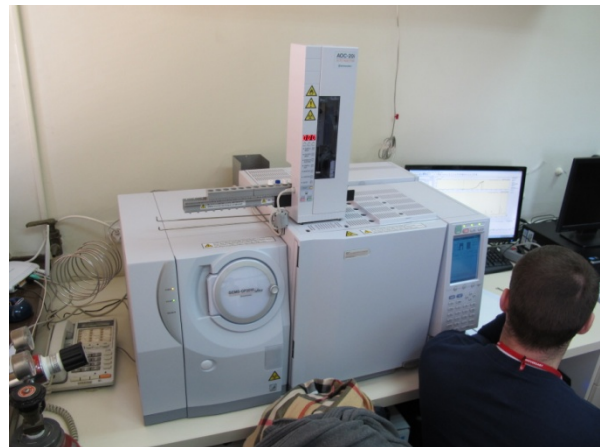
Fig 6. Installed Comprehensive GCxGC/MS
