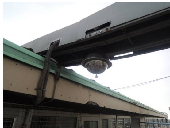
Fig. 12. Passive air sampler at the roof of FCUB
