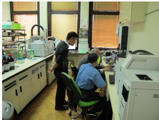
Fig. 8. Analysis of PCBs, fuel oil hydrocarbons and pesticide analysis using GCxGC-MS at FCUB.
